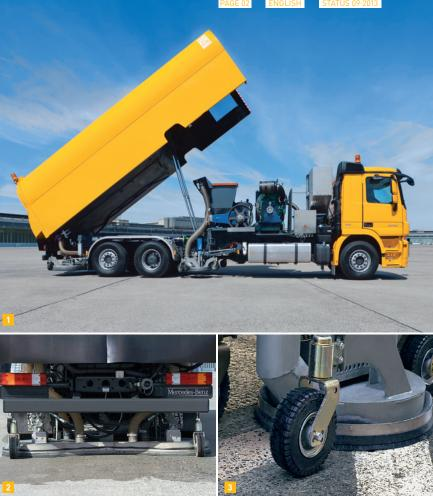
1 The tank and sound hood can be tilted hydraulically for maintenance purposes and for emptying the waste water tank. This allows easy access to all components - high pressure pump, boost pump, fan, cooler, extractor and auxiliary engine.
